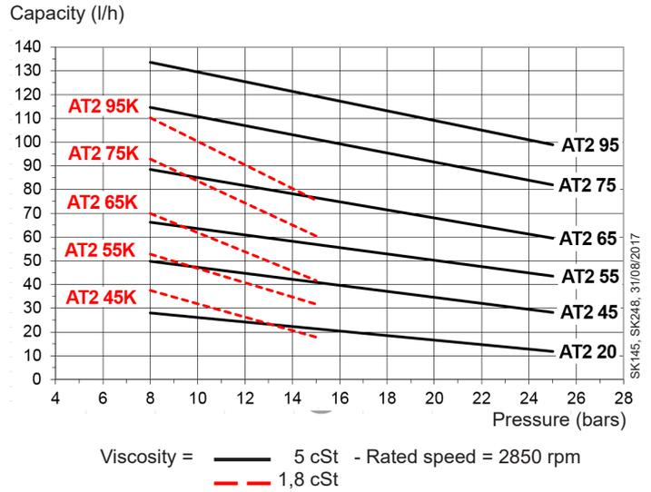
Data shown take into account a wear margin. Do not oversize the pump when selecting the gear capacity to ensure the optimum operation of the (NO) solenoid valve (switching low/high mode).
