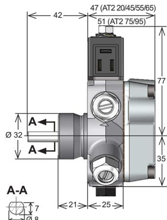
Inlet ① and Return ② with direct sealing for revision 6 models (sealing with washers can also be used)
