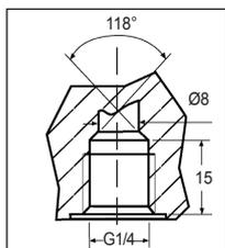
Inlet ① and Return ② with direct sealing for revision 6 (sealing with washers can also be used)
